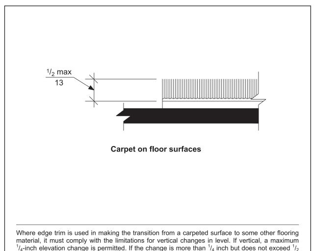
inch, a bevel is required with a maximum slope of 1:2.
