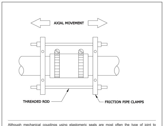
Although mechanical couplings using elastomeric seals are most often the type of joint to experience damage that is due to axial movement, this restraint requirement applies to changes in direction for all types of piping that exceed 4 inches in diameter.
