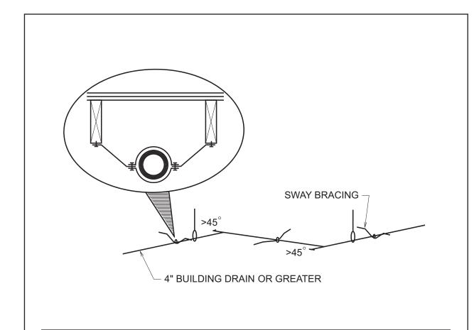
The maximum vertical and horizontal spacing between supports depends on the size and type of pipe. Supports must occur at frequent intervals for horizontal piping because of the potential for sagging. Although vertical piping typically requires support only at each story height, nonmetallic piping requires a mid-story guide or closer spacing.
