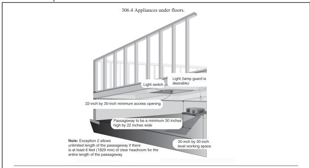
For both attic and under floor installations, a light fixture (luminaire) and a receptacle outlet are required at the appliance location for use during the service or repair of the equipment. The switch controlling the light fixture must be located at the entry to the passageway.
